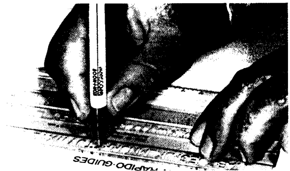
FIGURE 2.84 ■ Lettering guide template in use. Courtesy Koh-I-Noor, Inc.
